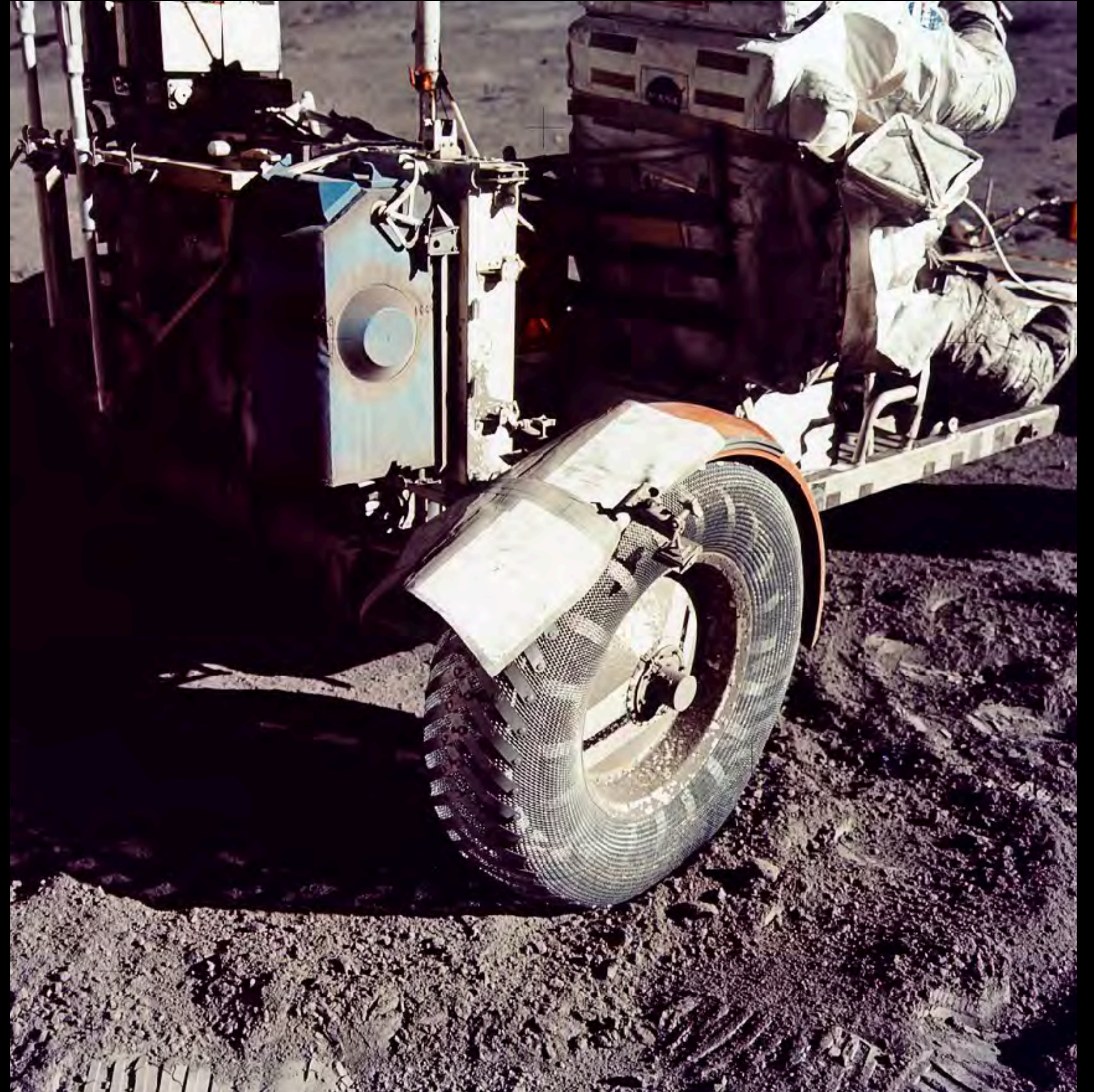
Duct tape fix on Apollo 17 mission
